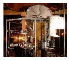
The NIST Watt balance: the vacuum chamber dome, which lowers entire apparatus, is visible at top. (CC BY-SA 3.0 Richard Steiner)
