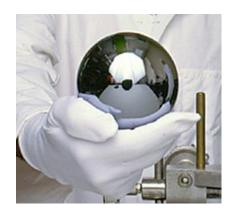
A 1-kg single-crystal silicon sphere for the Avogadro Project, used for measuring the Avogadro constant to a relative uncertainty of 2×10<sup>-8</sup> or less. (CC BY-SA 30.0 CSIRO)
